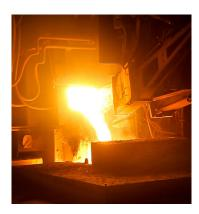
A heat-treatment furnace that uses electric current to control the temperature of a metal. Heat is supplied from electricity that arcs from the graphite electrodes to the metal bath. Furnaces may be either an alternating current (AC) or direct current (DC).
