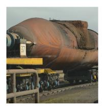
Cylindrical railcar lined with bricks and used for transporting the hot metal from the blast furnace to the steel shop (steelworks).
