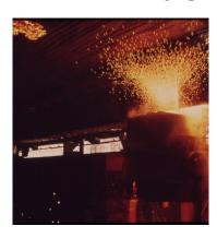
The basic oxygen furnace converts iron from the blast furnace into steel. When oxygen is blown over the molten iron in a BOF vessel, it combines with and removes carbon as carbon monoxide and carbon dioxide. Unwanted silicon, phosphorus and other elements are also driven off, while other impurities are combined with fluxes which are removed and then made into slag. The reactions in the BOF vessel creates heat, so ferrous scrap is added to cool it down.
