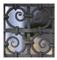
This is a type of iron, which unlike hard, brittle pig iron — such as is tapped from a blast furnace — is tough and malleable, allowing it to be forged and welded. It has a high tensile strength and is more corrosion resistant than steel. Wrought iron has a very low carbon content — lower than many steels — but importantly it has traces of manganese/sulphur/phosphorus/silicon-containing slag which give it a fibrous structure and which contributes to its desirable properties.
