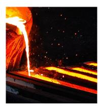
The process of making steel by heating the metal in the hearth of a regenerative furnace. Heat is supplied from a large, luminous flame over the surface, and the refining takes seven to nine hours.
