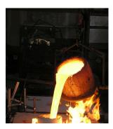
A process typically applied in a ladle furnace for alloying, deoxidation, desulphurisation as well as for temperature adjustment prior to casting of quality steels.
