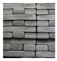
An ingot is a mass of metal obtained from casting liquid steel into a mould. The resulting ingot - a semi-finished product - is typically then hot rolled or forged.
