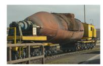
Cylindrical railcar lined with bricks and used for transporting the hot metal from the blast furnace to the steel shop (steelworks).
